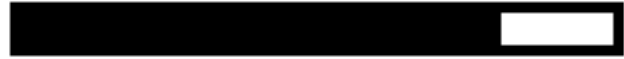
Figure 2. A barcode control bar. The placement of the white region indicates the orientation of the barcode. The size of the white region relative to the size of the black region indicates the 'level' of the barcode, which establishes the barcode's dimensions and bit density.
