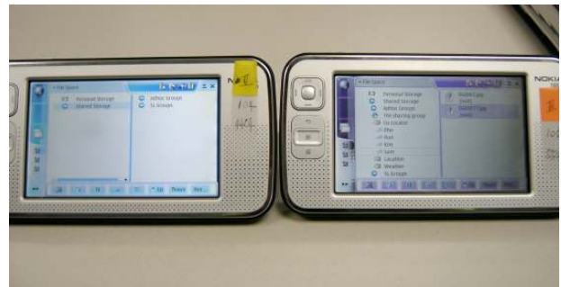
Figure 5: Right-side device is browsing Left-side device's local folder
