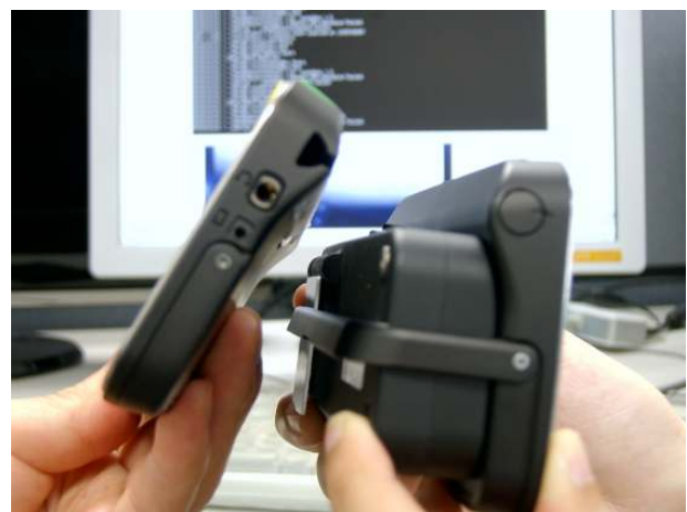
Figure 2: Right-side device with Sensor Board read the RFID tag on the left-side device
